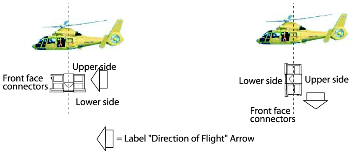
Figure 204: KANNAD 406 AF-H installation
